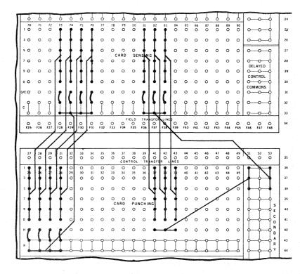
In this example; Card Columns 73 - 76 are wired to Reproduce in Card Columns 25 - 28; Card Columns 81 - 83 are wired to Secondary Reproduce in Card Columns 37 - 39.
