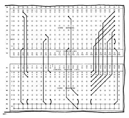
Because of the individual Position sockets in the columns of Card Sensing and Card Punching; partial split and transposed wiring for Reproducing, such as shown in this and the following example, is possible.
