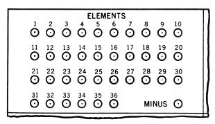
As the machine proceeds through a Program, one of these indicators will light each time the related Input or Constant Value is used in a Program Step as VI or V2. When the machine stops or is stopped during a run, none of these indicators will be lit as the stoppage occurs at the conclusion of the Step.
