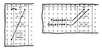
The transposed reproduction of information sensed from one set of columns in a card to another set in the same card can be performed on a selective basis by card control.
