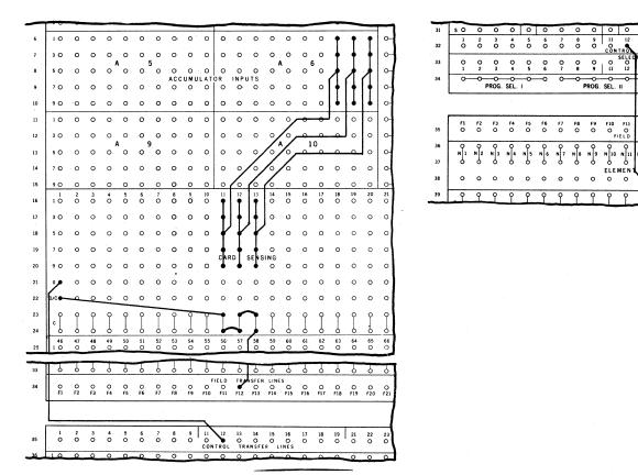
A zero in a card column outside the Input Value card field is used in this example. A field consisting of Card Columns 11 - 13 is wired to Accumulator Columns 3 - 1 of Input A6. The zero in Card Column 1 is punched when this value is negative.
