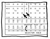
A Selector Pick Up is connected directly to a Selector Hold socket. The related Selector will assume the Select position when the current to the Computer is turned On. It will remain in the Select position as long as the Computer current remains On.
