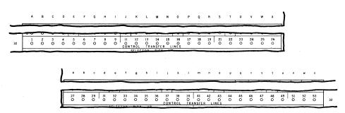
These 48 sockets, numbered 1 through 53 (the numbers 10, 20, 30, 40, and 50 are not used) are the terminals on the Constant & Program Panel for the direct connection between this panel and the Input & Output Panel. Each terminal here is related by number to its corresponding terminal on the Input & Output Panel.
