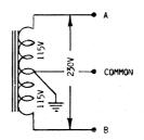
Two wires of a three wire system with 115 Volts from center wire to each outside wire with 230 Volts across the outside wires. Center wire is for voltage regulator connection only.
