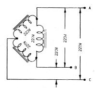
Three wires of a three wire system are used, with 220 Volts across each pair of wires. Wires must be capable of carrying 30 Amperes. Computer current is 21 Amperes, plus or minus 2 Amperes on each leg.
