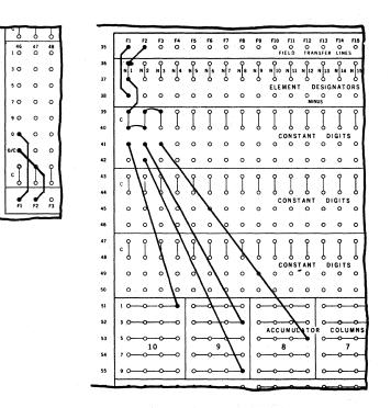
In this example, the Constant Value 145, Element N1, is to enter Accumulator Columns 10 through 8, as either negative or positive depending on whether the 0 in Column 46 is punched or not.
