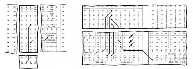
One Selector whose Pick Up is impulsed by card control, is used to initiate a Selector Hold operation for another Selector. The Selector Hold wiring from the Selector Pick Up of the Selector to be Held is routed through the Select side of the controlling Selector.
