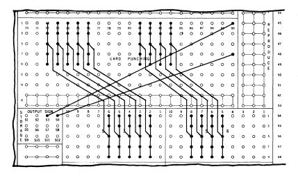
The output of Unit S3 is wired to Card Column 72 - 76; its Storage Output Sign is wired to the 1 position in Card Column 90. The output of Unit S4 is wired to Card Columns 81 - 84; its Storage Output Sign is wired to the 7 position of Card Column 90.
