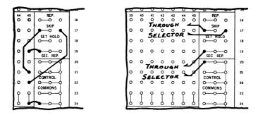
The Skip Cycle and Set Hold functions are equally effective for the Secondary Reproduce as they are for Reproduce.
