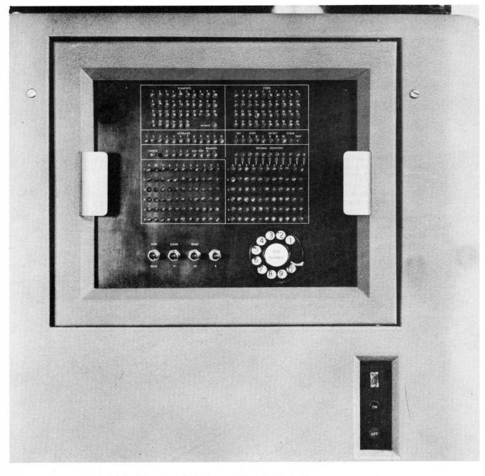
Included in this view of the Program Test Panel is the Computer On-Off Switch Panel at the lower right corner.
