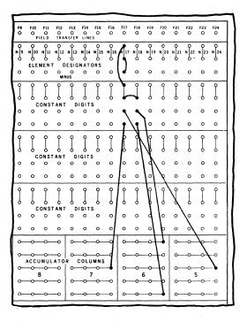
In this example, the value 525, Element N17, is to enter Accumulator Columns 7 through 5 as a Constant Negative Value. The connection between the Minus socket and the Element Designator socket in the Element Designators section causes that Element always to be negative.
