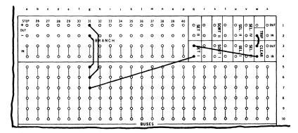
Branching may be from a Program Step to an Operational Step, from an Operational Step to an Operational Step as shown in this example. This illustrates possible wiring at the end of a Program. A Double Branch connects the final Program Step, No. 31 in this case, to Set I, Set I is wired to Clear, Clear is wired to Trip to conclude the Program.
