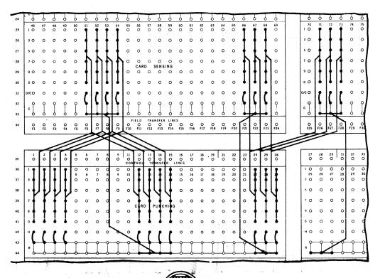
Y-Wired and Inversion connections for Reproducing can be made.
