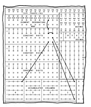
When one or more of the digits of a Constant Value is zero, no connection is made from the Accumulator Columns section to the Constant Digits section. With no connection made to the Constant Digits section, Call (C) wiring for zeros is not required.
