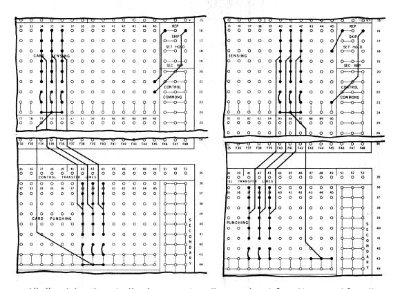
With the wiring shown in the above examples, the Reproduce information sensed from the card containing the Reproduce control punching will be punched in the card containing the control punching and into all following cards until the next Reproduce control punching is sensed. The Reproduce information is retained because of the H (Hold) connections in the Card Punching section.
