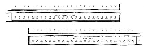
These 48 sockets, numbered F1 through F48, are terminals for direct connections between the Input & Output Panel and the Constant & Program Panel. There is a similar set of 48 sockets bearing the corresponding numbers of the Constant & Program Panel.
