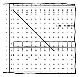
The "I" in Accumulator Column 1 of Storage Output S1 is wired to the 1 socket of Card Column 46. Any emission from the 1 socket of S1 will cause punching in position 1 of Column 46. This emission occurs for both the 1 and 2 of the 90-Column Numerical code.
