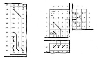
In this example, either the initial Program Step or the Trip is impulsed according to the control punching sensed from individual cards.
