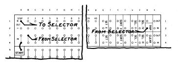
In this example, the connection from the Start to the initial Program Step for the calculating operation and the Trip is routed through a Selector.
