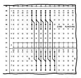
Shown above are typical connections from Storage Output to Card Punching. With these connections, the value in Intermediate Storage is delivered during a Set operation to the Punching Setup Section as an Output Value.
