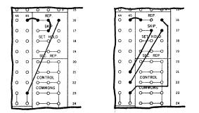
When punching is not desired in the card from which Reproduce information is sensed, the Skip Cycle operation is used in conjunction with the Reproduce control. Skip Cycle may also be used within a group to prevent punching in selected cards.
