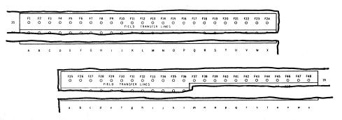
These 48 sockets, numbered F1 through F48, are the terminals on the Constant & Program Panel for the direct connections between this panel and the Input & Output Panel. Each terminal here is related by number to its corresponding terminal on the Input & Output Panel.
