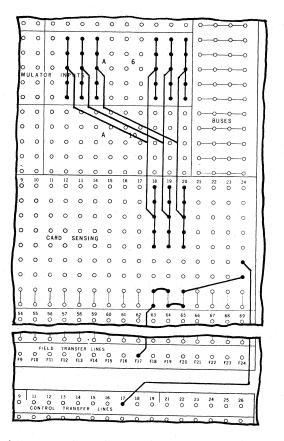
One card field, Card Columns 18 - 20, is connected to two sets of Accumulator Columns 3 - 1 and 9 - 7. The two inputs are controlled by one negative sign identification; a separate negative control cannot be applied to both sets unless that control wiring is routed through Selectors.
