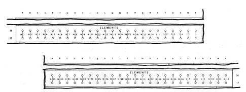
The 48 vertical rows of two common sockets each within this section (A-x,16&17) represent the Elements to be used and the Result to be obtained in the Equation for each Program Step. The two sockets in each vertical row are interconnected at the rear of the panel to serve equally.
