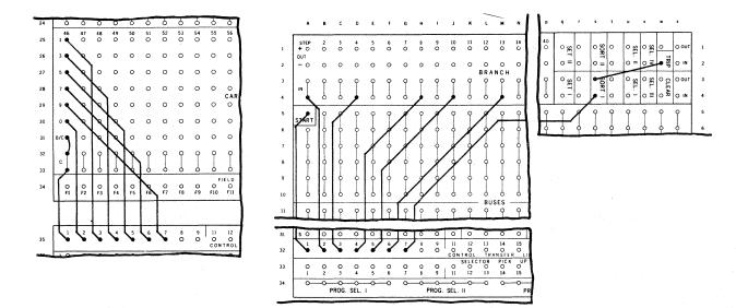
In the above illustration, Card Position Selection is being used as a means of branching from Start to one of five different Program Steps or to an Operation.
