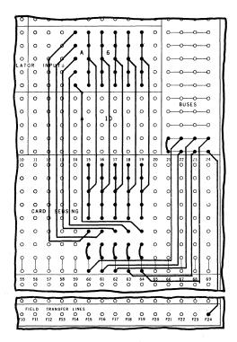
The zero positions of a card field are used for added capacity. The five sockets (1, 3, 5, 7, & 9) for each card column are connected on a socket-for-socket basis to the related sockets (1, 3, 5, 7, & 9) for Accumulator Columns 2 through 6 of Accumulator Input A6.
