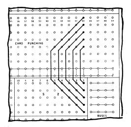
The wiring to Card Column 65 from Accumulator Column 1 of Storage Output S2 is completely transposed; 1 to 9, 3 to 7, 5 to 5, 7 to 3, 9 to 1.
