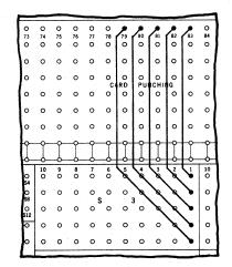
The wiring from Accumulator Column 1 of Storage Output S3 is split so that the emissions from the individual sockets will register as "1's" in Card Columns 79 - 83. Note that the 9 socket of Accumulator Column 1 of S3 will emit for all even numbers.
