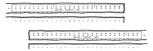
These 48 sockets, numbered 1 through 53 (the numbers 10, 20, 30, 40, and 50 are not used) are also terminals for direct connections between the Input & Output Panel and the Constant & Program Panel. There is a similar set of 48 sockets bearing the corresponding numbers on the Constant & Program Panel.
