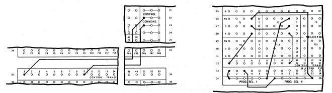
The individual Program Selects may be de-activated and reused repeatedly during the same Program. If the connection between a Program Select and the Selector Pick Up or Pick Ups to which it is connected is broken, the related Program Select will drop out ready to be reused in the same Program.
