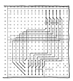
The zero positions of a card field are used for added capacity in this example. The 1 - 9 sockets in Accumulator Columns 5 - 1 of Storage Output S5 are wired to Card Columns 56 - 60 on a socket-for-socket basis. Each socket in Accumulator Column 6 of S5 is wired to a zero socket in Card Columns 56 - 60.
