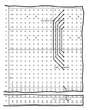
The wiring of Card Column 13 to Accumulator Column 8 in Accumulator Input A6 is completely transposed; 1 tc 9, 3 to 7, 5 to 5, 7 to 3, 9 to 1.
