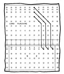
The "1" sockets of Accumulator Columns 1, 2 and 3 of Storage Output S2 are wired to three different sockets in Card Column 61. An emission from a 1 socket will be punched in the card column position to which it is wired.
