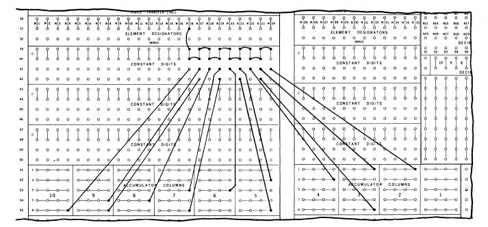
In this example, the value 987654321 is to enter Accumulator Columns 10 through 2. This Constant Value is to be Element N16.
