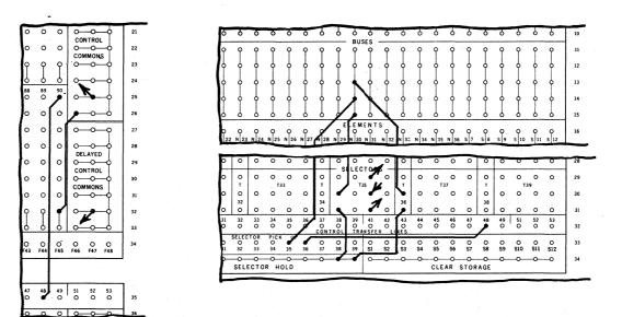
A Selector Hold operation is to be initiated by Card Control. However, the Control Commons and the Delayed Control Commons are to be used for other purposes than Selector Hold.
