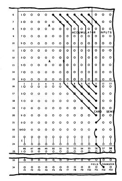
The wiring of Card Column 11 is split so that the individual positions, including the zero, will register as "l's" in Accumulator Columns 1 through 6.
