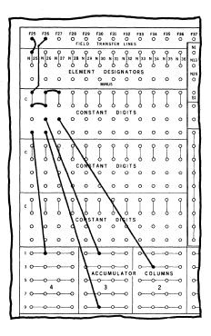
A Constant Value can be either zero or a significant digit value according to the absence or presence of control punching.
