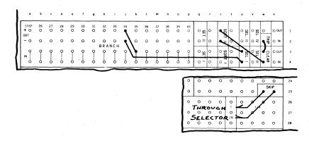
This is a typical example of the use of the Program Controlled Skip Cycle. On Program Step 34, when the Result is positive, the Program is to proceed to Program Step 35. When the Result is negative; the Program is to end, all punching is to be withheld from the card, the card is to be segregated into the Front Card Receiver, and Intermediate Storage is to be Cleared.
