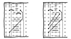
To prevent Output Values from clearing during a Skip Cycle operation, the Set Hold is used.
