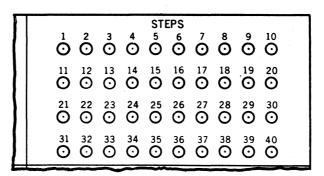
The 40 indicators in this section headed "Steps" are related to the 40 Program Steps. The Program Step to which each indicator is related is printed on the panel just above that indicator. These are the actual Program Step Numbers; not necessarily the sequence within a particular Program.
