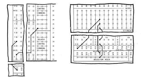
A Selector Hold operation is initiated by Card Control. The wiring from the Selector Pick Up is routed through the Select side of the Selector to be controlled to the Selector Hold.
